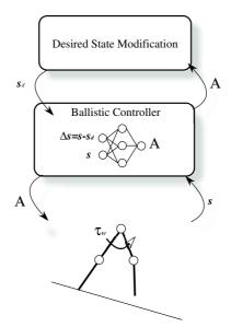
Figure 5: Layered controller with neural network
