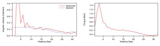
(a) the angular velocity of hip joint at the moment of heel strike in each step
